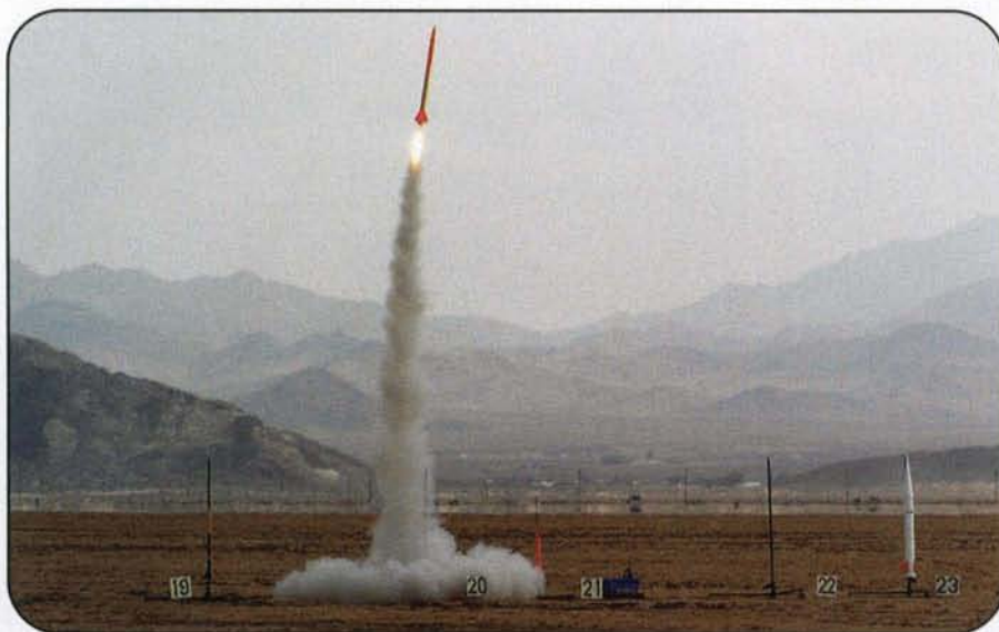
A high-power rocket lifts off at Lucerne Dry Lake. Launchers have sliding rods that aim rockets toward the sky, to land away from the observers. (Photo by KØOV)
