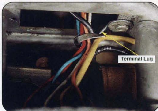
Photo 12. Secure the lugs in place with the solder lug as shown (see step 21).
