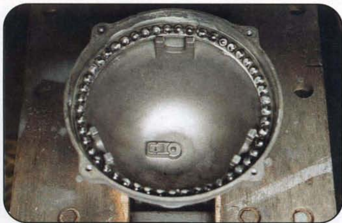
Photo 19. The bearing is set in place, flange up, and the sockets are engaged by the ring-gear mating protrusions (see step 38).
