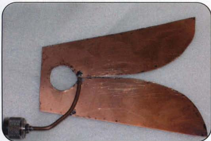
Photo E. The finished homebrew 1- to 6-GHz Vivaldi.
