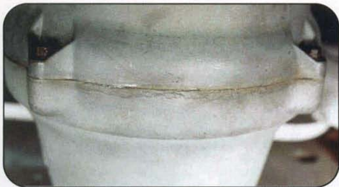
Photo 21. There is no appreciable gap between the two halves of the housing (see step 43).
