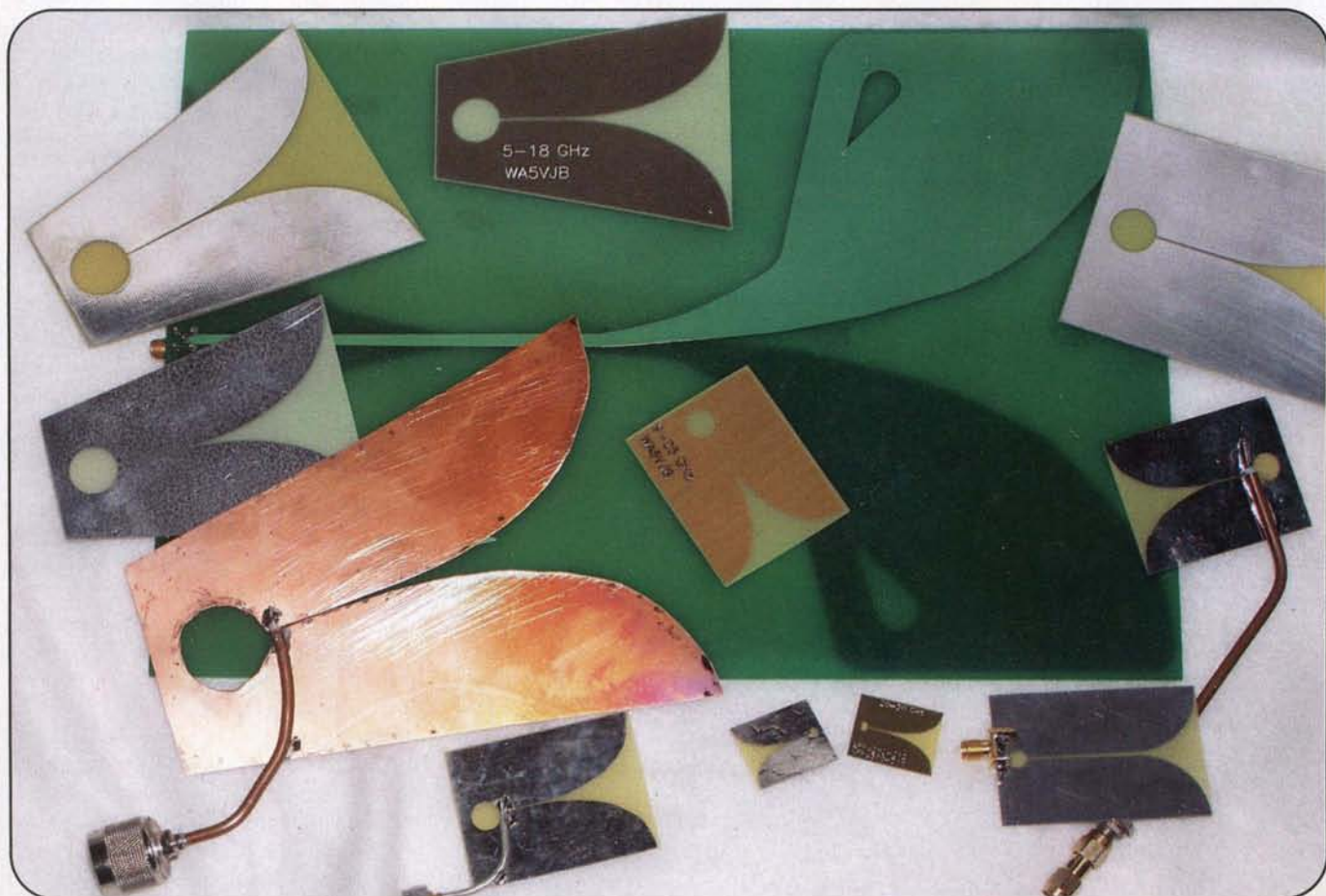
Photo A. Vivaldi antennas from 900 MHz to 35 GHz. (Photos and figures by the author)
