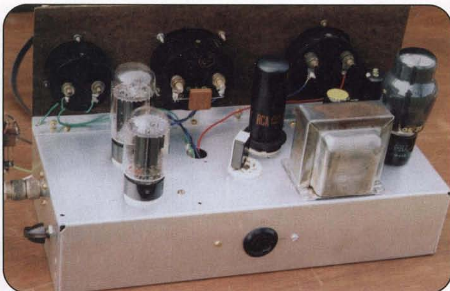
Photo C. Rear view of the transmitter: 6L6GC bi-push finals on the left, metal 6L6 oscillator tube, Heising modulation choke, and 6L6G modulator tube on the right.
