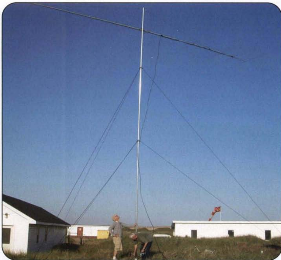
Photo 4. Robby Robertson, VY2SS, loaned us this custom 8-element M 2 6-meter Yagi on a 40-foot boom which he had used for his CY9SS 2005 St. Paul 6-meter DXpedition.
