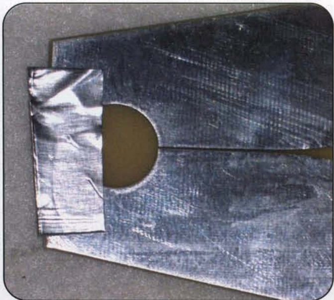
Photo G. Changing the high-frequency matching.
