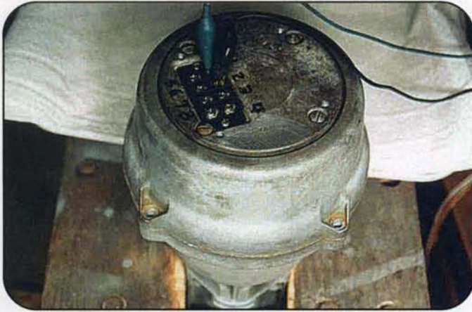
Photo 1. Turn the rotor upside down with the "Vee" of the mast bracket facing away from you, securing the rotor in a vise (see step 1). (All photos by the author)
