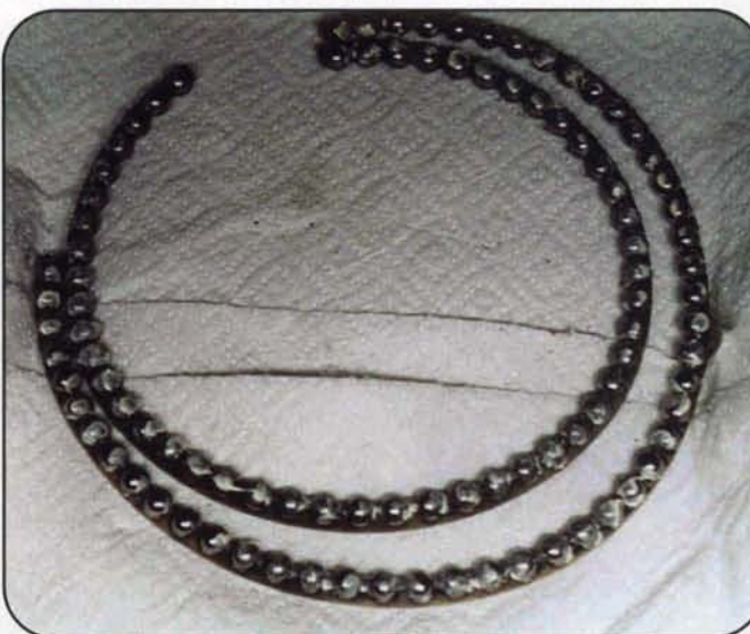
Photo 18. Lightly lubricate the bearing sets (see step 37).
