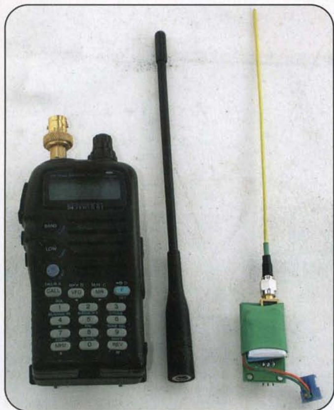
The BeeLine 433-MHz transmitter and quarter-wavelength antenna are dwarfed by a handie-talkie. The SMA antenna connector is a factory option. (Photo by KØOV)
