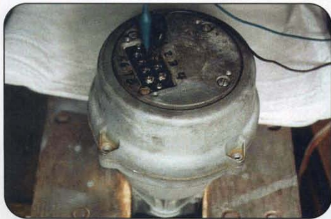
Photo 22. Prepare to align the bolt holes in the housing halves before installing the four housing screws (see step 44).
