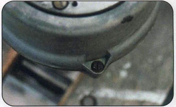
Photo 2. Remove the four #12-24 screws that hold together the upper and lower halves of the rotor (see step 2).
