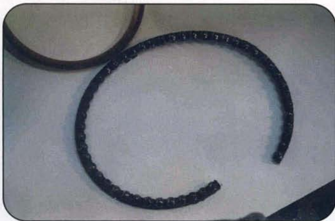
Photo 5. The bearing set, one of two. This one is caked with dirt and grease (see step 5).
