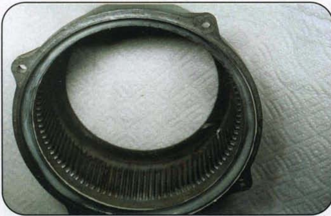
Photo 3. Lift the brake housing (or retaining ring for the TR/CD rotors) straight up away from the rotor. The plastic spacer may come off and remain inside the brake housing (see step 3)
